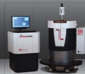
PPMS ® DynaCool ™ Base: 1.8 K - 400 K Oven: 300 K - 1000 K Dilution Refrigerator: 0.050 K - 4.0 K
